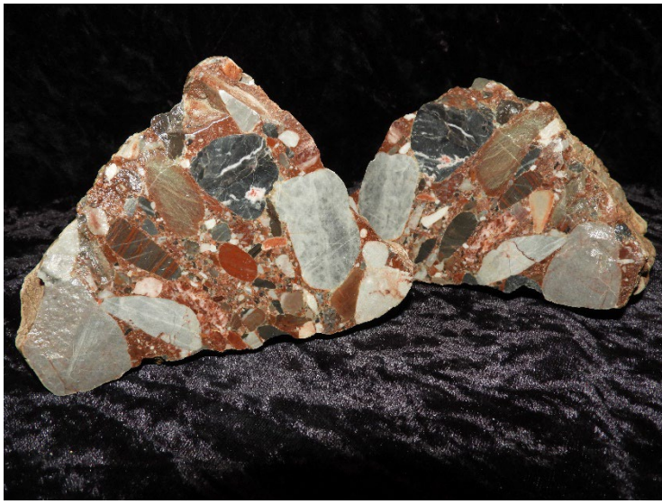
Polished Potomac Marble sample showing inclusions.
